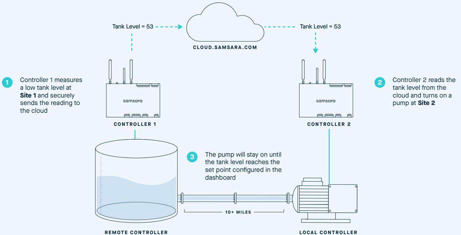
Remote Variables: Using remote variables, Central Texas can collect data points at one location and use them to control outputs at a second location.
