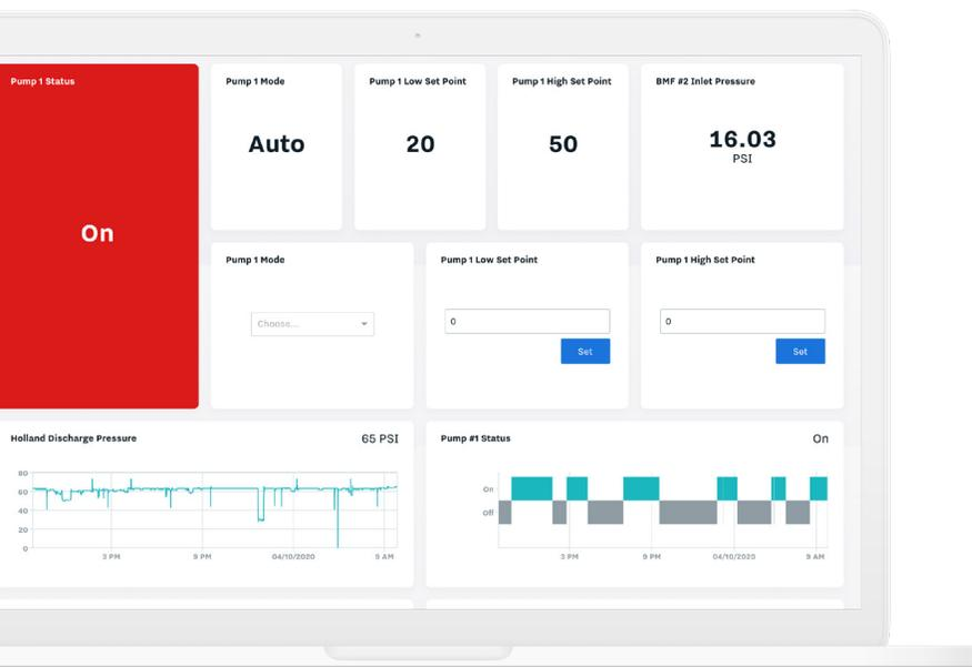
**REAL-TIME MONITORING** to keep a close eye on pressures and flows, catching leaks and line breaks before they lead to service interruptions
